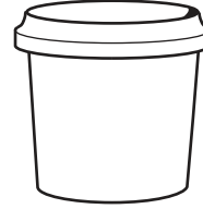
paint pot Ø70 at top 70 high Ø60 at bottom
